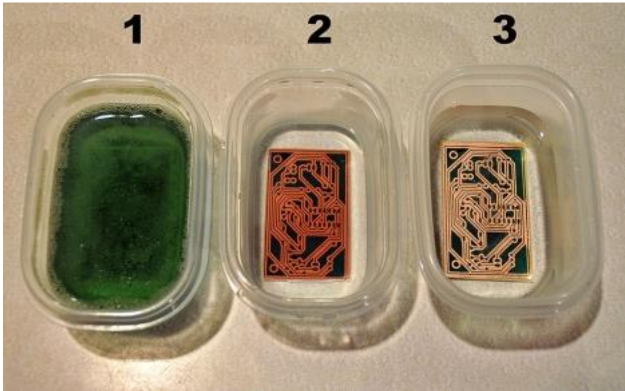
Ferric chloride etching of copper boards
