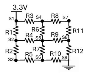
$$R_1 = R_2 = R_6 = R_7 = R_{11} = R_{12} = 100\Omega$$
