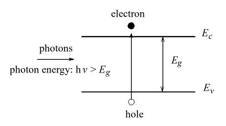
•  $E_g$  can be determined from the minimum energy (h v) of photons that are absorbed by the semiconductor.
